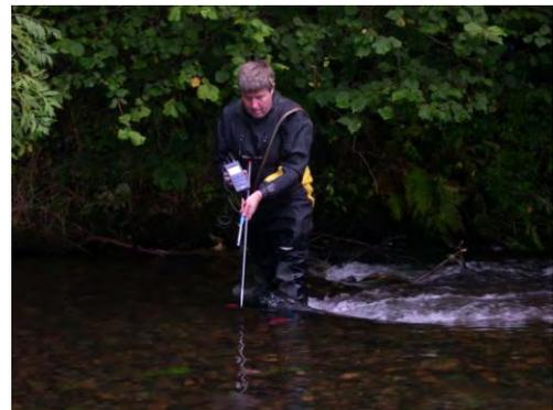
Figure 2: Taking redox measurements
